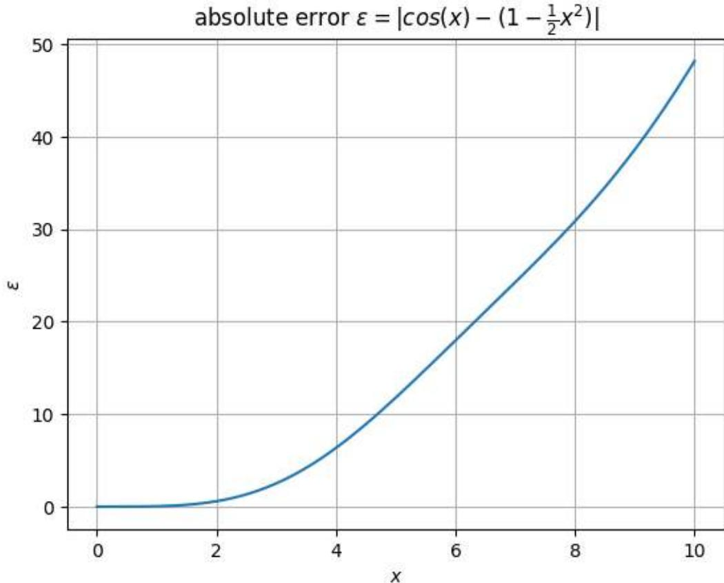
If we plot this on a double-logarithmic scale, we can verify the power 4, in  $x^4$ , as follows
