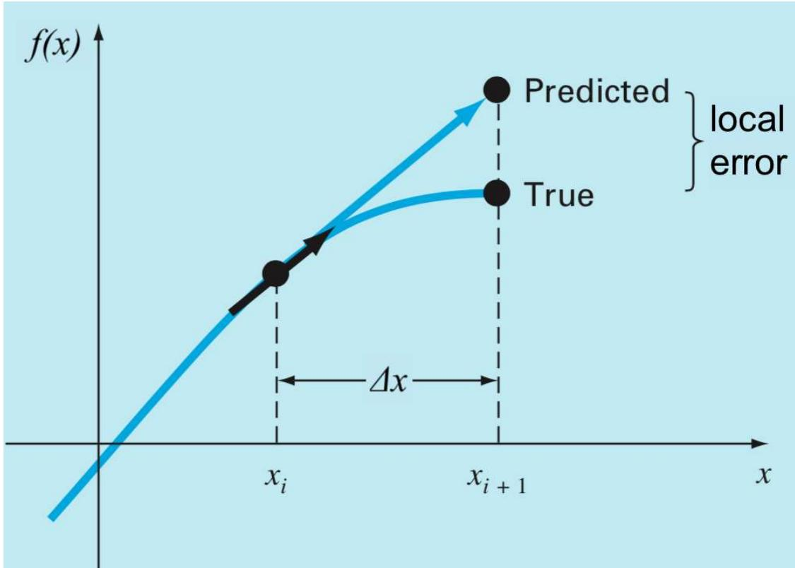
So the error due to the *truncation of the Taylor series* in  $f(x + \Delta x)$  is for small  $\Delta x$  proportional to  $\Delta x^2$  (since  $\Delta x^3$  is even smaller and can be neglected).
