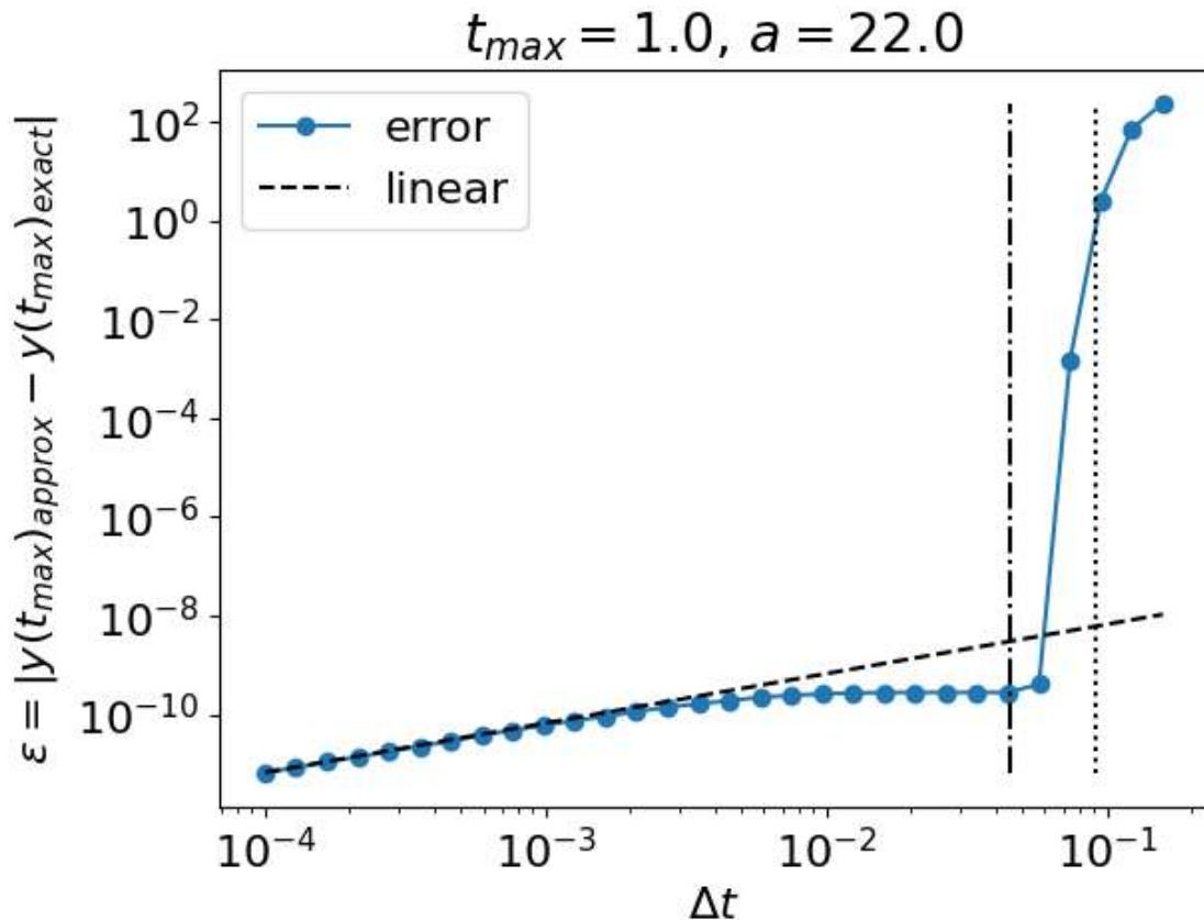
The explicit Euler algorithm becomes *unstable* for  $a\Delta t > 2$  (second, dotted, vertical line). It shows *oscillatory behaviour* for  $a\Delta t > 1$  (first vertical line).
