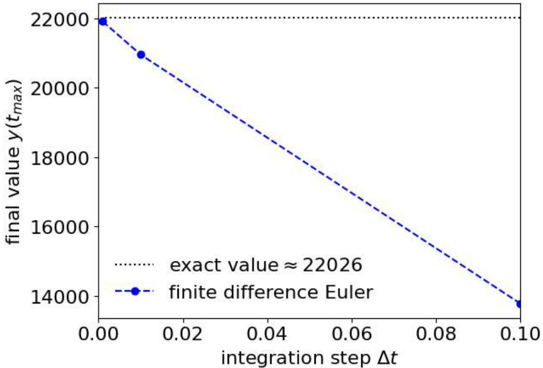
The error between the finite difference scheme and the Euler method is the difference between the blue and black curve.
