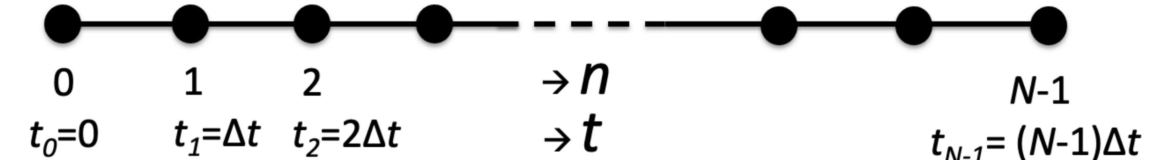
$$t_0 \rightarrow t_1 = t_0 + \Delta t \rightarrow t_2 = t_0 + 2\Delta t \rightarrow \dots \rightarrow t_{\max} = t_{N-1} = t_0 + (N-1)\Delta t.$$
