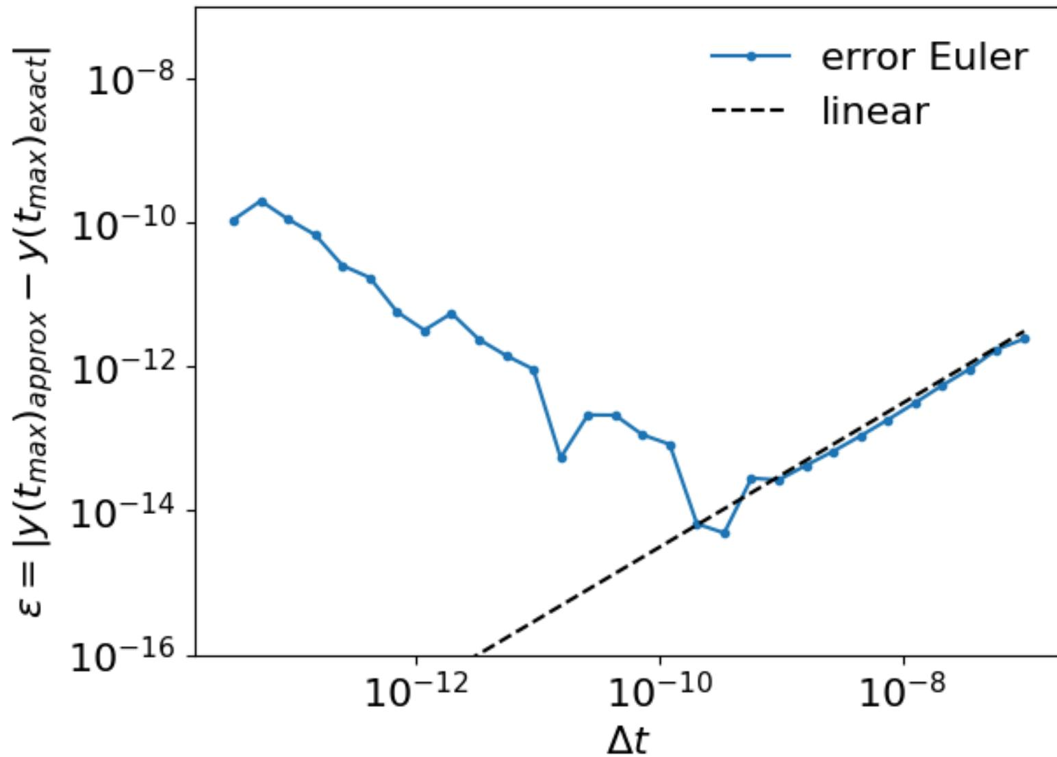
From  $\Delta t \lesssim 10^{-9}$  the error does not decrease any more with smaller time-step. The reason: limited accuracy of the 64 bit floating point number is reached. For  $\Delta t \approx 10^{-10}$  the error in the calculation  $\epsilon \approx 10^{-13}$ .
